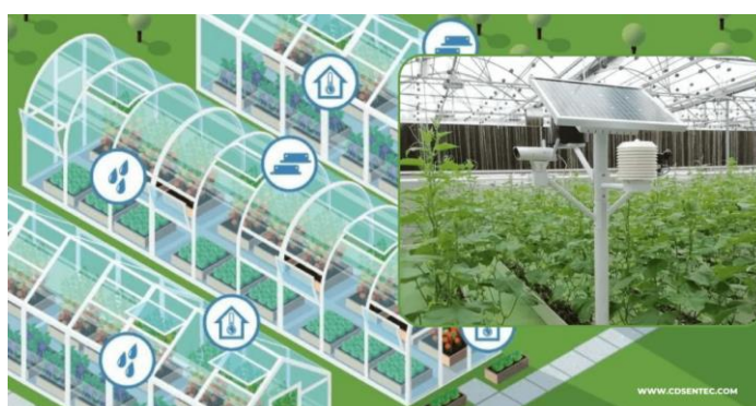
Figure 1. Smart greenhouse equipped with IoT sensors monitoring temperature, humidity, light, and soil moisture for precision flower production.
