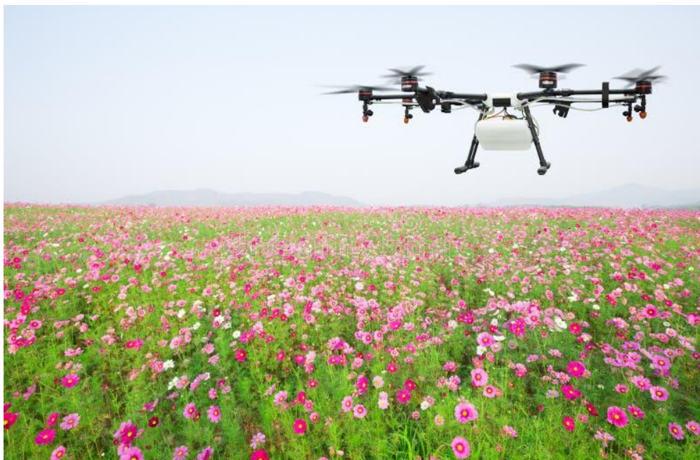
Figure 4. An agricultural drone monitoring a flowering field—precision aerial technology enables site-specific spraying, mapping, and eco-friendly crop management.
