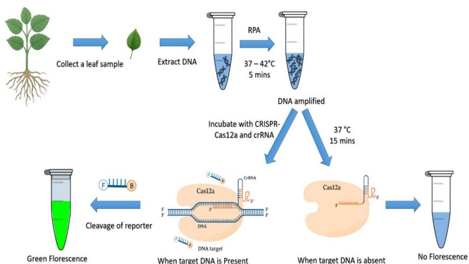
FIGURE: The workflow diagram for the RPA-CRISPR/Cas12a detection assay. Following recombinase polymerase amplification of the target DNA, Cas12a binds to a sequence-specific crRNA and activates its collateral cleavage function by binding the amplified product. When
